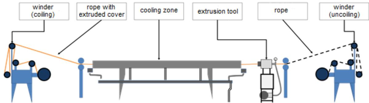
Figure 3 Scheme of tubing-extrusion for fibre ropes
