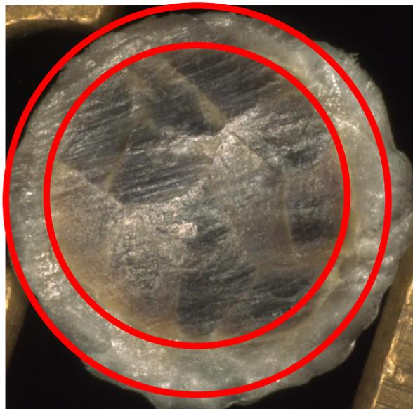
*Figure 6 Cross section of a braided fibre rope with braided cover*
