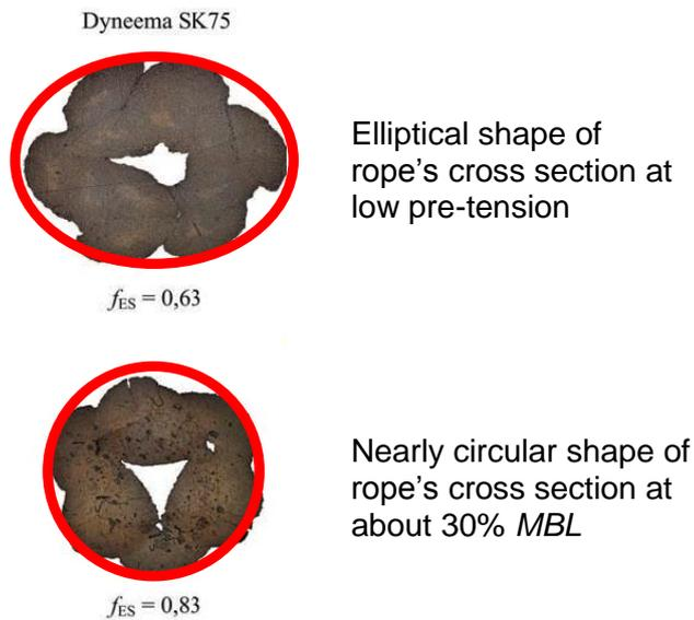
*Figure 5 Effects occurring in the cross section of fibre ropes under varying load*
