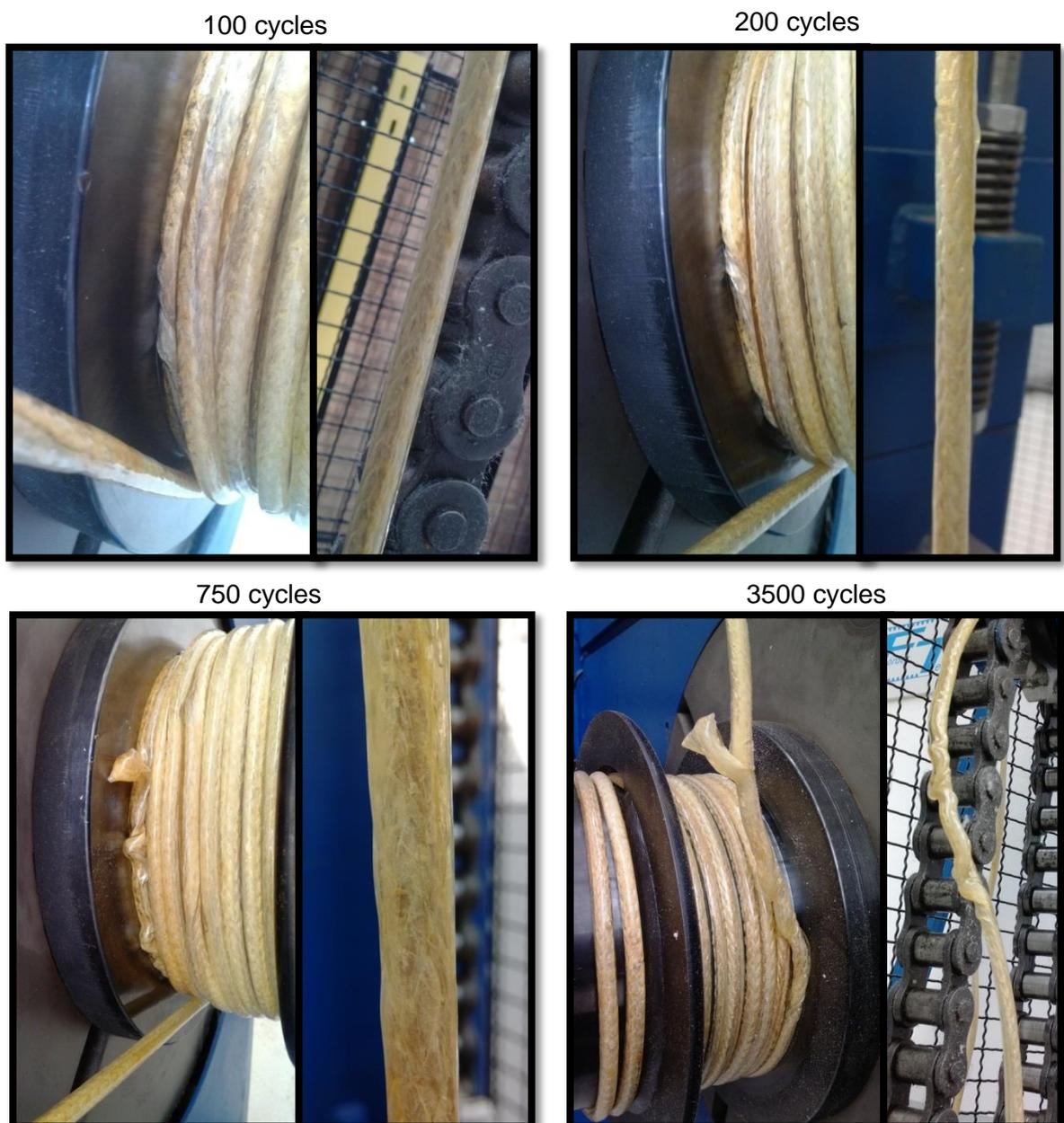
Figure 7 Winding tests on a fibre rope with a polyurethane cover (tubing-extrusion)
