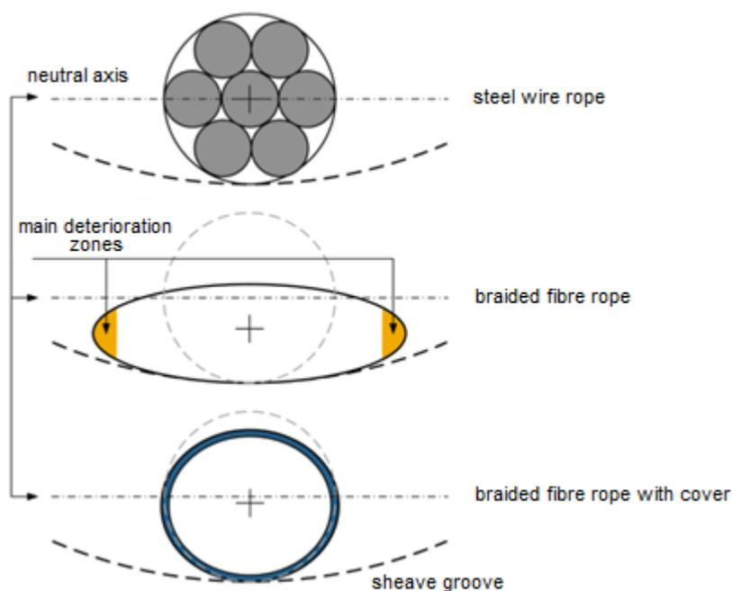
Figure 1 Dimensional stability of steel wire ropes and fibre ropes
