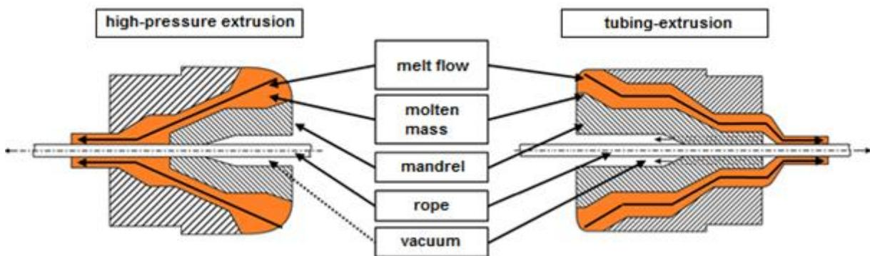
Figure 2 Tools for extrusion of cover layers according to [1]
