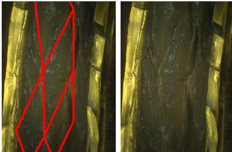
*Figure 8 Tubing-extrusion layer separated from the core rope*
